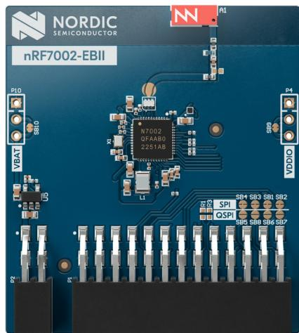
The nRF7002 Expansion Board II (nRF7002 EBII) is a plug-in board designed to add advanced Wi-Fi 6 connectivity to Nordic's nRF54 Series Development Kits. It provides everything needed to start developing Wi-Fi applications on the nRF54L platform. The board connects through a dedicated expansion header and uses the DK's nRF54L multiprotocol System-on-Chip (SoC) as the host for the nRF7002 Wi-Fi Companion IC.
